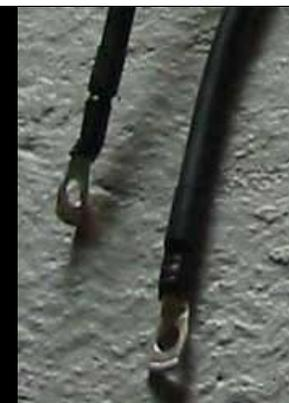
I crimped the wires and soldered as well for extra conductivity (But crimping will suffice if you don't have a soldering iron).
