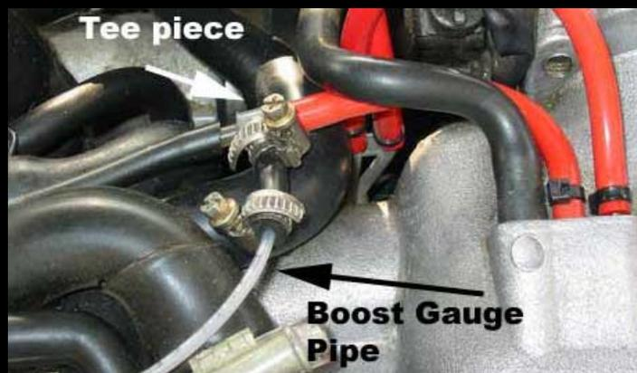
For earlier cars MY93-MY96 there are three ports coming from the manifold all are in use, generally the centre one is used for a boost gauge, and usually the centre pipe has a T-piece (which is unused) attached to it a couple of inches from the manifold, a good place to put in your new boost pipe.
