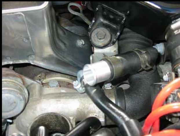
**4.** The particular Dumpvalve I fitted was a Forge Motorsport unit.
