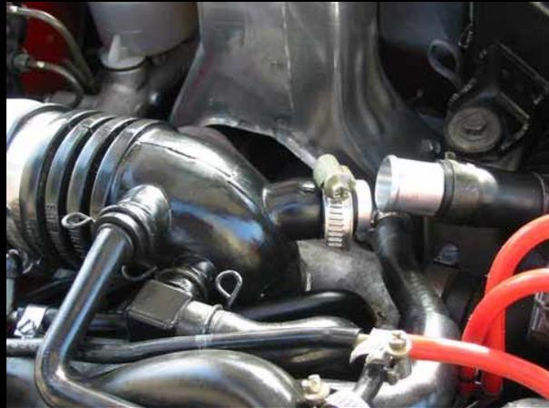
**6.** All that is left is too fit the Red silicone hose to the Aluminium adaptor and then fit the Dumpvalve to the hose.
