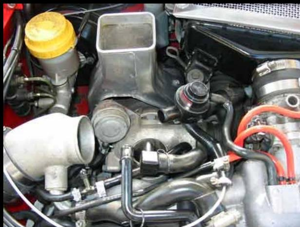
2. Next remove the large Air pipework from the Air intake and turbo outlets. This now leaves the original dumpvalve accessible.
