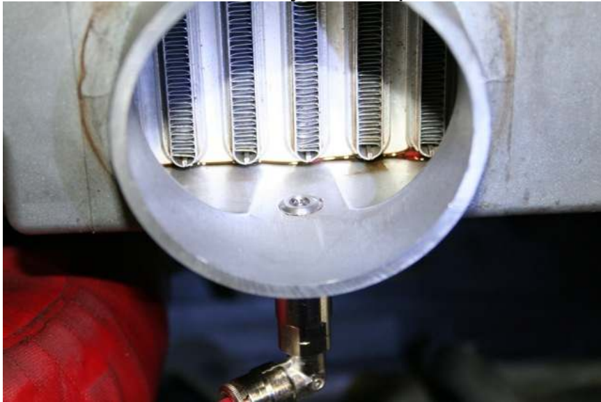
Nozzle mounted at the outlet of the factory intercooler. Note the slight projection of the nozzle tip into the airflow.
